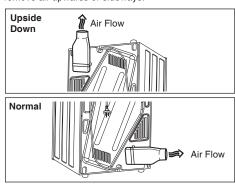
Inlet and outlet points need clear airflow to prevent overheating, so ensure there is adequate ventilation. (i.e. open window or external door.)
