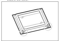
**5.** Release the locking system to remove the internal glass panel.
