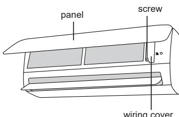
2. Make the power connection wire go through the cable-cross hole at the back of indoor unit and then pull it out from the front side.
