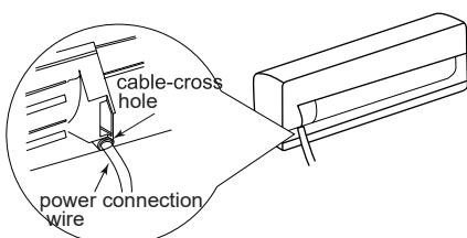
3. Remove the wire clip; connect the power connection wire to the wiring terminal according to the color; tighten the screw and then fix the power connection wire with wire clip.
