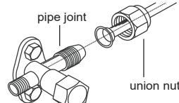
4. Tighten the union nut with torque wrench by referring to the sheet below.
