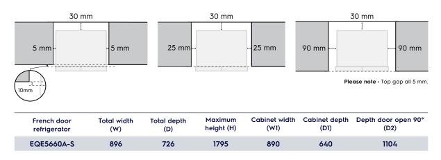
Please note! Dimensions to be used as a guide only. All customers MUST refer to the user manual supplied with the product for detailed installation instructions. © 2022 Electrolux S.E.A PTE. LTD. E\_DIM\_EQE5660A-S\_Oct22
