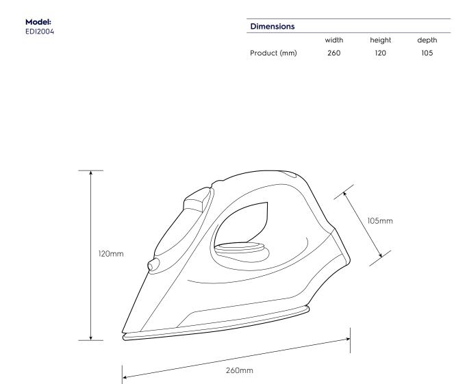
Please note! Dimensions to be used as a guide only. All customers MUST refer to the user manual supplied with the product for detailed installation instructions. © 2022 Electrolux S.E.A PTE. LTD. E\_DIM\_EDI2004\_Apr22
