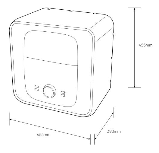
Please note! Dimensions to be used as a guide only. All customers MUST refer to the user manual supplied with the product for detailed installation instructions. © 2021 Electrolux S.E.A PTE. LTD. E\_DIM\_EWS30IDX-DWM\_Jun21
